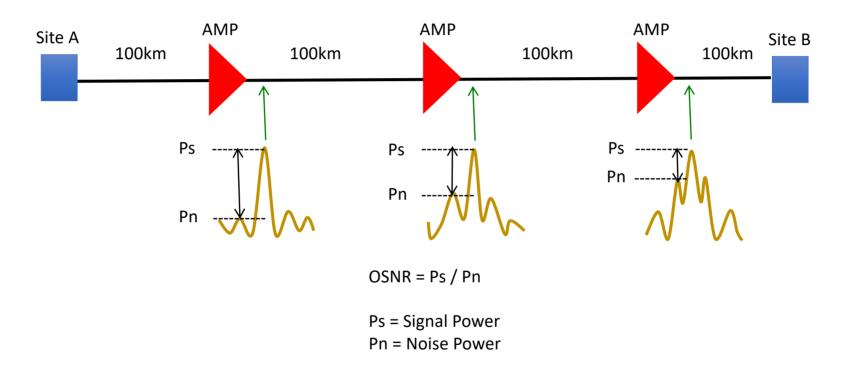
The noise power increases with each added amplifier stage, decreasing the OSNR. If the OSNR gets too low, then the signal is not recoverable once it get to Site B.
