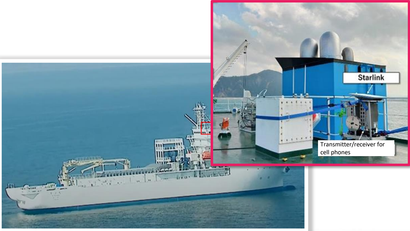
Cell Phone base station on board using Starlink
